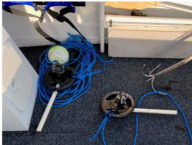
Figure 5.1. BRUVS setup, showing the float and rope, 5 kg weight, attached GoPro and PVC arm – bait bag not shown. Photo by Hika Rountree.
