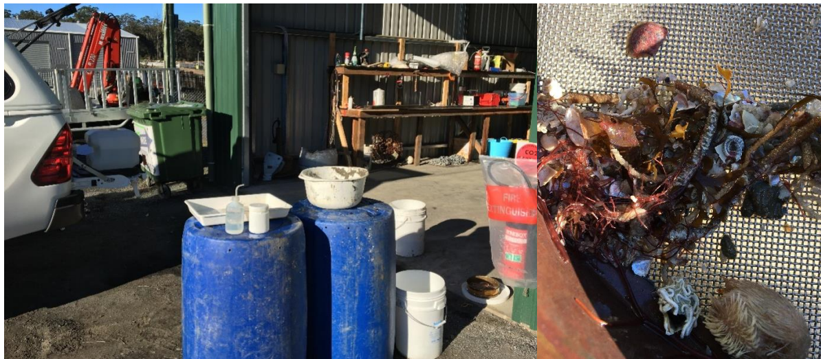
Figure 4.3. Sampling of benthic macroinvertebrate samples, showing (left) sieving set up – including tray for sieves, basin for rinsing (on top of blue drums), ethanol container (on vehicle tailgate) and (right) benthic macroinvertebrates on a 1 mm sieve, with a heart urchin at bottom right and a pteriid bivalve in the upper part.
