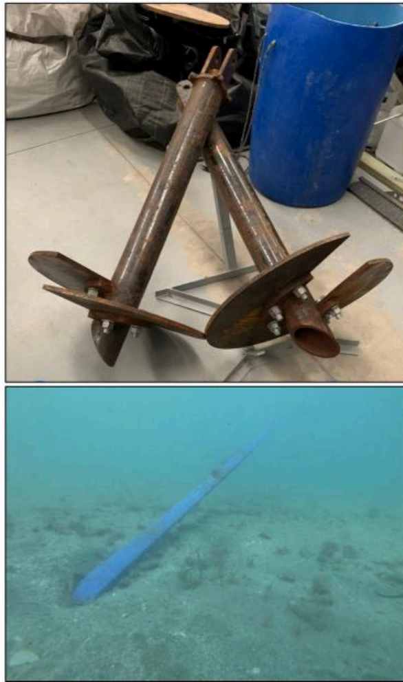
Figure 16: The top shows screw anchor with plate and bottom shows screw anchor inserted into benthic floor. (Source: NSW DPI, 2023)
